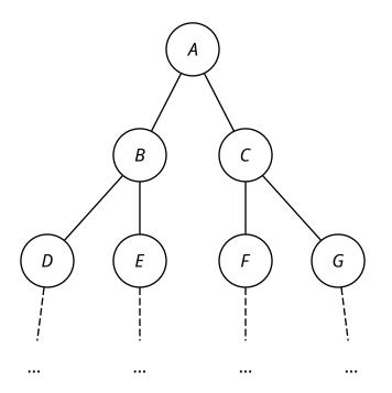
Let's first compute the resistance of the whole circuit. Since the branches going  $A \rightarrow B$  is symmetric with the branch going  $A \rightarrow C$  The resistance of this whole circuit is equal to half the resistance of the following circuit.
