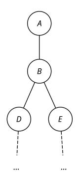
The resistance of this sub-circuit is 1 + R where R is the resistance of the whole circuit. So we have that  $R = \frac{1+R}{2}$  and hence R = 1.
